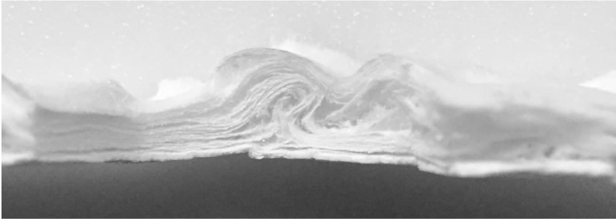
Introducing the IW Tremont MultiDensity™ filter disk. This exciting new product is a 100% borosilicate binderless glass microfiber filter which demonstrates several layers of density along with a unique surface formation that speeds and optimizes filtration. These filter disks can handle sample preparation tasks typically considered too challenging for other analytical filter products. This unique product bridges the gap between macro and micro analytical filtration.
