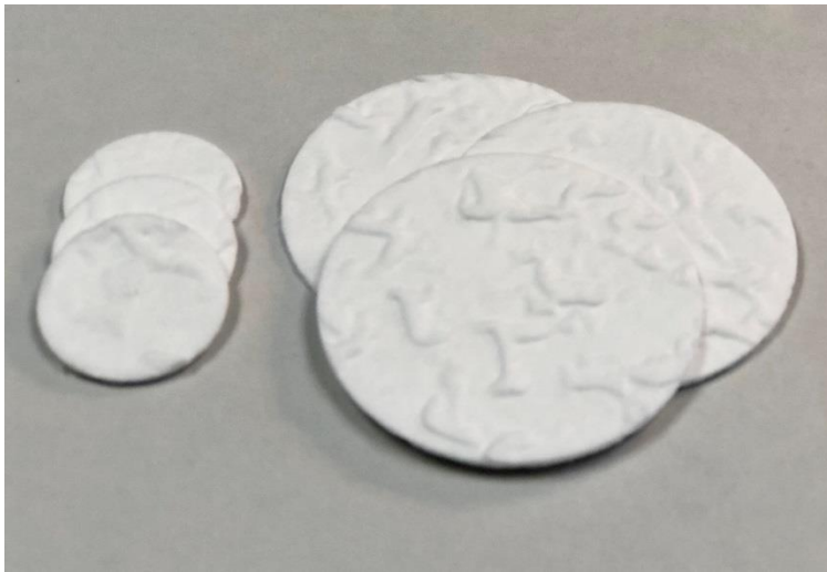
The wavy pattern of the MultiDensity™ Filter Disk easily distinguishes the sample introduction side.
